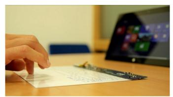
The surface is both lightweight and flexible, meaning OEMs can integrate it into protective covers or provide larger desktop touch zones. It can also act as a super-slim keyboard or detect handwriting or sketches via modified pen, with touch latency of just 12 milliseconds.
