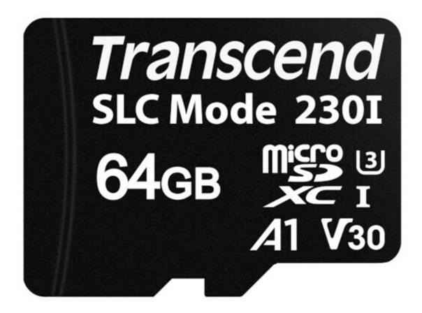
The cards carry both A1 and V3 badges, meaning they can be used to install Google Android applications with a minimum write speed of up to 30MB/s, or good enough for 4K video shooting. First introduced back in 2017, so far pseudo-SLC caching has not been used in other memory cards. The USD230I range uses 3D TLC NAND memory, necessitating the need for pSLC caching to boost writing performance.
