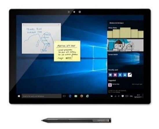
The stylus supports both Microsoft Pen Protocol (MPP) and the Wacom Active ElectroStatic (AES) protocol, making it compatible with devices with a broad range of devices, from the MPP-support **Microsoft Surface** laptops to the AES-supported **Lenovo Thinkpad** tablets. Switching between protocols simply involves holding both side buttons.
