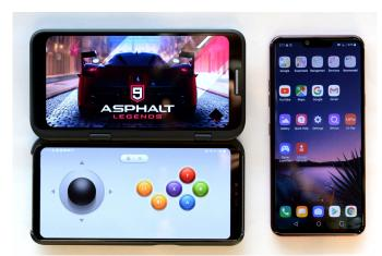
Revealed at MWC 2019, the second screen is designed to look like a cover case. It offers a 6.2-inch OLED panel for "double the viewing, gaming and multitasking experience," as well as hinge able to rotate a full 360-degrees. Connectivity takes place via proprietary wifi chipset allowing very short-range and high-bandwidth communication between the display and the phone, while Pogo pins hook the Dual Screen in place and provide power from the phone battery.
