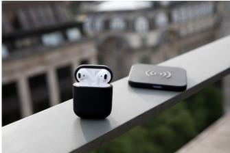
On September 2017 Apple announced a Qi-compatible AirPods case-- something that, a year later, is still to actually materialise. Enter the PowerPod case, a silicon case for the AirPods case promising an end for cable-based charging. It has a Lightning plug on the bottom connected to a Qi charging coil on the front, and allows charging on any Qi-enabled charging pad.
