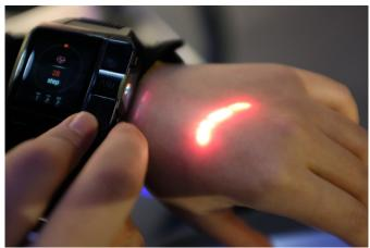
The Asu wins no awards for sleek design, since it is far bulkier than other wrist-worn devices of its ilk. As one might imagine the extra bulk comes from the projector, which the company says augments the 1.54-inch display with 480 x 854 resolution projections. Users can interact with the projections via touch, making for a larger surface than standard smartwatches. For instance, one can tap on projected digits to store a phone number or draw on the projection with a finger.
