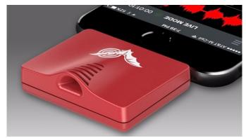
The device is, essentially, a highly sensitive microphone with a Lightning connector. One simply needs to plug it into the iPhone, iPad or iPod Touch before firing up a free companion app. The microphone picks up ultrasonic bat calls, while the app adds amplification (making them audible to human ears), displays an interactive spectrogram and even determines the kind of bat making the call in question.
