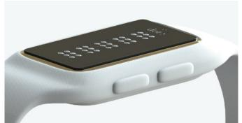
Instead of a display the Dot features a series of pins spelling 4 Braille characters at a time by rising and falling at custom speeds. The devices connects to smartphones via Bluetooth and provides regular smartwatch features (such as watch, alarm, messenger and navigation) as well as act as a Braille eReaders.
