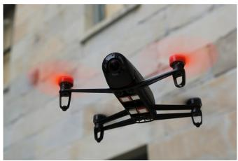
Designed for flights both inside and outside the house (with styrofoam bumpers providing bump protection), the Bebop carries a 14MP 1080p camera complete with 180-degree fish-eye lens. A combination of sensors and image processing ensures smooth video, even when the drone is flying through choppy airs.
