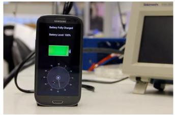
A Microsoft Think Next symposium demo has a near-empty nanodot battery inside a Samsung Galaxy S4 fully charging up in all of 30 seconds. The company also claims the batteries "withstand thousands of charge/discharge cycles, prolonging battery life expectancy considerably."
