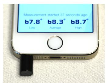
The Thermodo carries a highly-sensitive sensor inside a tiny package, and works together with a companion app. Once plugged in iOS or Android devices it measures air temperatures, with the app providing readings and graphs.
