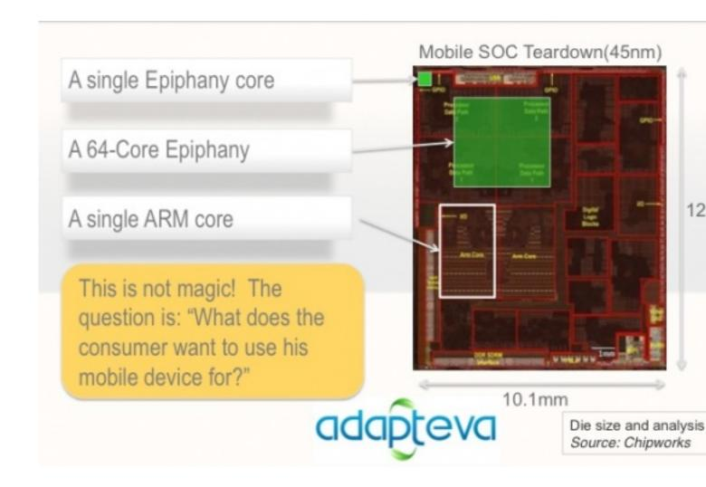
The design can scale to up to 4096 cores (which would run on 64W), but Adapteva's current focus is on mobile applications. The company says an Epiphany 64-core accelerator would also be quite small-- 8mm square.
