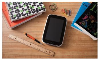
Currently available as a reference design, the Studybook has most of the features one expects in a device for younger customers. It is a 7" (1024x600) Atom-powered tablet running on either Android 3.0 or Windows 7 with 1GB of RAM. Storage ranges from 4-32GB to a 128GB SSD.
