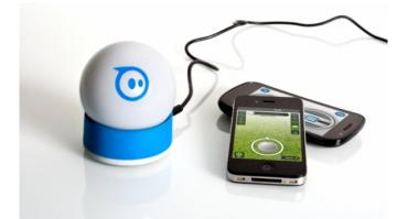
The Sphero looks unassuming-- it is basically a palm-sized white plastic ball. Inside, however, are a "smart robot" (with a gyroscope, compass and accelerometer), a multi-coloured LED (producing "thousands of colours") and a Bluetooth radio. Powering it is a rechargeable battery carrying up to 1 hour of juice.
