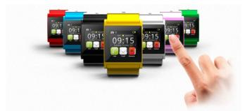
The I'm Watch has a 1.55" 240 x 240 curved TFT touchscreen, 64MB RAM and 4GB of storage, and uses a version of Android 1.6. Tethering to a mobile phone via Bluetooth, it handles caller ID, speakerphone (calling Dick Tracy!) and music streaming duties, and at launch will work with iPhone and Android devices.
