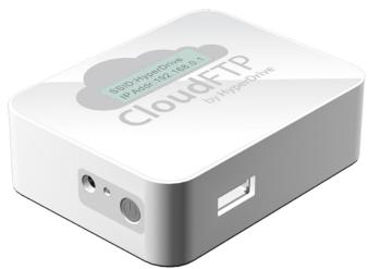
It not only creates an ad-hoc wifi network (working independently of the internet or other existing wifi networks) to share connected USB data, but also connects automatically to online cloud-based storage services such as iCloud, Dropbox and box.net.
