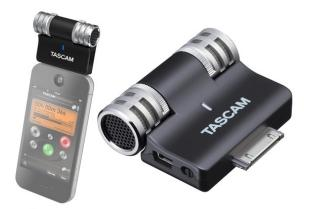
It carries x2 condenser microphones (the same found in Tacsam's DR-series recorders) and plugs into Apple dock connectors. The microphones are adjustable over 180-degrees, with uni-directional elements arranged in an AB pattern for detailed stereo imaging.
