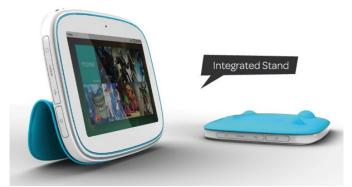
It has a 7" capacitative multitouch display, a 1.2GHz Cortex A8 processor and 1GB of DDR3 RAM, making it upgradeable to either Honeycomb or Ice Cream Sandwich Android versions.
