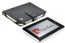
It runs last year's Android (version 2.2) and comes in a 7" form factor, complete with a Cortex A-8 1GHz processor, 512MB of RAM, 4GB of internal storage (expandable via Micro SD cards) and built-in wifi.
