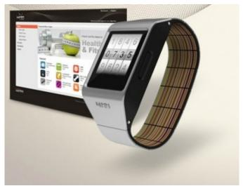
The result of a partnership with Foxconn, the preview kit (known as the WIMM One) is a 1" slab packing a reflective colour touchscreen (160 x 160 resolution), wifi, Bluetooth and GPS radios, vibrate motor, accelerometer and magnetometer.
