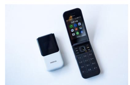
With the Nokia 2720 Flip, HMD promises a simple and reliable device within the much loved flip form factor. Built out of tough polycarbonate, it features big hardware buttons paired with a 2.8-inch internal display and a 1.3-inch external display. Operation is just like it used to be. The external display shows call details and various notifications, and one can answer calls by opening the phone. Once ready, the user simply snaps the phone shut.
