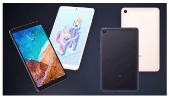
As an upgrade on the previous Mi Pad 4 has a slimmer design even if the display gets something of a downgrade from 2048 x 1536 resolution to 1920 x 1080. The internals however get a boost, with 3/4GB LDDR4x RAM, 32/64GB internal storage (expandable via microSD card) and f/2.0 13MP front-facing camera.
