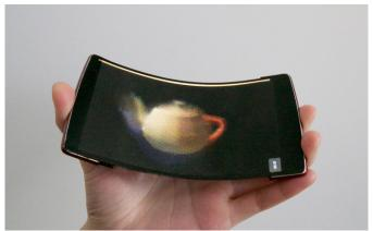
Seen in early prototype form, the Holoflex features a novel display with a microlens array on top. The lenses disperse light in multiple directions to create 3D images multiple users can simultaneously see, all without need for head tracking or 3D glasses.
