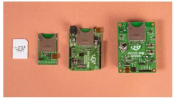
Created by ex-Apple and Google engineers, the Electric Imp card looks very similar to standard SD cards. It carries a wifi 802.11b/g/n radio, a Cortex M3-based processor and software-controllable I/O pins.
