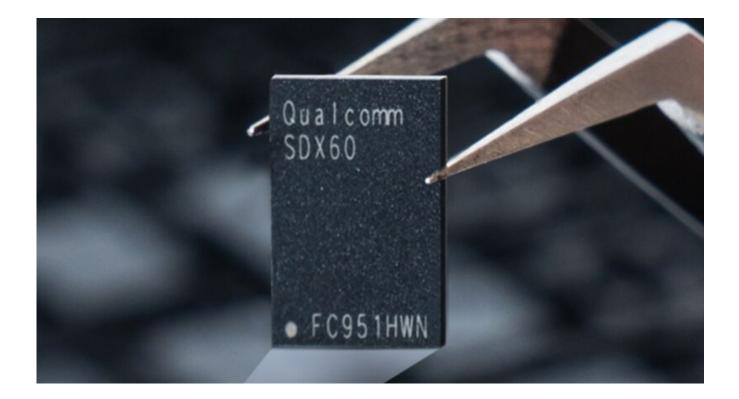
As a result, the Snapdragon X60 supports mmWave and sub-6 using frequency division duplex (FDD) and time division duplex (TDD), allowing smartphones to uplift 5G performance using fragment spectrum assets. Such capabilities, Qualcomm says, make it a solution able to enhance performance and capacity for operators worldwide while increasing average 5G speeds in mobile devices.
