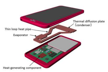
Fujitsu develops a liquid cooling system for thin mobile devices of smartphone and tablet variety, making it possible for CPUs and other devices to run cooler while avoiding hot-spots inside devices.
