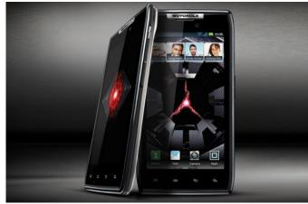
Motorola says the Droid Razr is the thinnest 4G LTE smartphone around, with a 7.1mm-thick body and a 4.3" Super AMOLED 960x540 touchscreen. Inside is a 1.2GHz dual-core processor, 1GB of RAM and an 8MP rear-facing camera capturing video at 1080p resolution.
