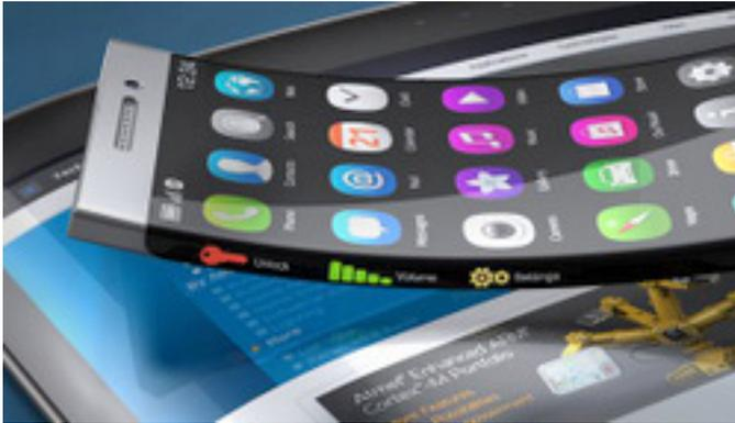
Atmel Corporation is in beta with **XSense**, a flexible touch-panel technology that you can roll it up).
