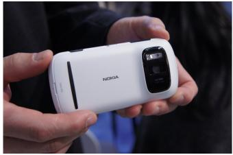
PureView technology uses "oversampling"-- taking image data from 7 neighbouring pixels and combining it into one pixel to generate a single 2/3, 5 or 8MP image (technically not 41MP, but still impressive for a mobile device).
