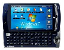
It's basically a PC inside a compact (measuring 125mm x 61mm x 19.8mm) design, with a 1.2GHz Intel Atom Z600 processor, 1GB of LPDDRR400 memory and 32GB of eMMC storage.
