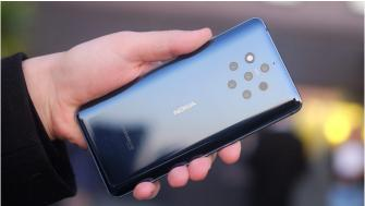
The 5 cameras share the same specifications, since each features a 12MP sensor and an f/1.8 lens. Two of the cameras shoot in colour, while the other three are in monochrome. To snap a photo, the cameras shoot at different exposures at the same time, before the phone merges all the image data into a single, ultra-detailed shot. Nokia even claims the individual cameras can shoot multiple exposures on their own, adding even more data to the final image.
