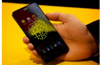
Launched at Mobile World Congress 2014, the Blackphone is a collaboration between Spanish mobile maker Geeksphone and security developer Silent Circle. It looks like a regular 4.7-inch smartphone with a 2GHz quad-core processor, 2GB RAM 16G storage and an 8MP rear-facing camera but runs on "SmartOS," a modified Android version promising to "keep communications private without extra effort."
